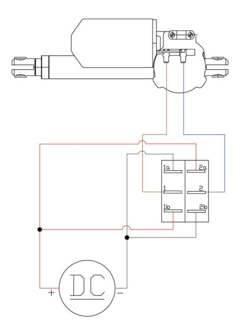
The selection of power supply and the use of fuses and/or electronic current override protection depends on the actuator model and the application. For specific actuator connections, direction of travel relative to the polarity and for other information please refer to the datasheets, user manuals or contact our Technical Support team.
