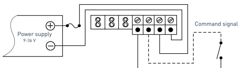
4 EXTERNAL INPUT SIGNAL CONNECTION 4-20 mA
