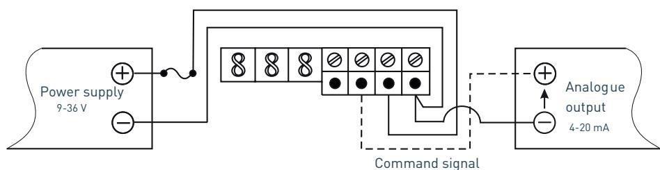
5 TWO WIRE TRANSMITTER INPUT CONNECTION 4-20 mA
