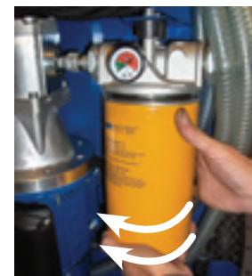
Fig. 6: Loosen the filter by turning it counterclockwise
