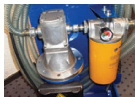
Fig. 12: Checkpoints for any air being sucked in
