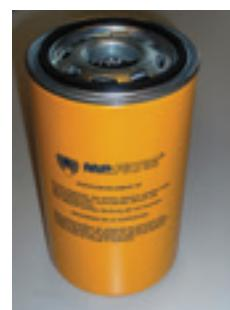
Fig. 9: Oil filter element to be replaced
